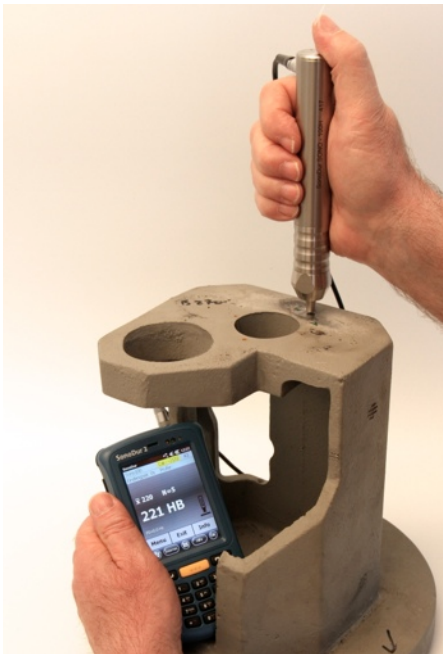
Fast and precise hardness tester the new SonoDur2 on GGG50 cast iron and remote control via PC
